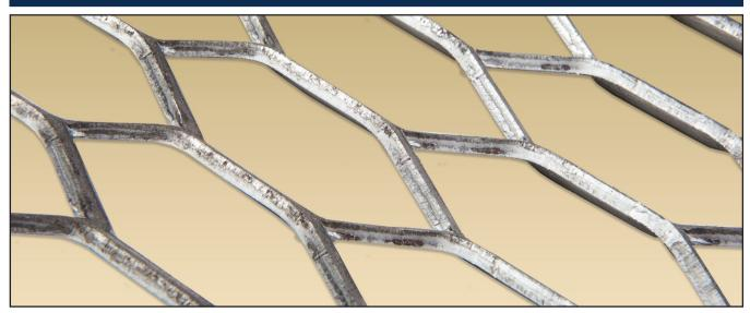
The manufacturing process that produces expanded grating is similar to that of expanded metal. The difference is in the thickness (gauge) of the strand. Expanded grating has a thicker strand gauge which affords it load bearing characteristics and therefore lends itself to a wider variety of applications.
